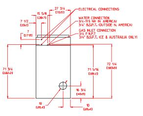
Specifications in parentheses are metric equivalents. \* For single-phase (1ø) dryers use 1 motor: 1 hp drive/fan. For three-phase (3ø) non-reversing dryers use 1 motor: 1 hp drive/fan and for three-phase (3ø) reversing dryers use 2 motors: 1 hp fan and 1/2 hp drive.
